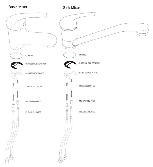
Screw on mounting nuts and fasten firmly with a tube spanner to secure the mixer
