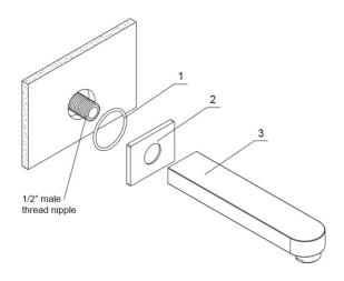
Insert the O Ring (1) into the base
