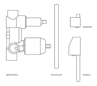
Mount the mixer body into the wall cavity securing it to the mounting stud. The distance between the rear mounting surface and the rear of the wall cladding and the cut out are as per the above
