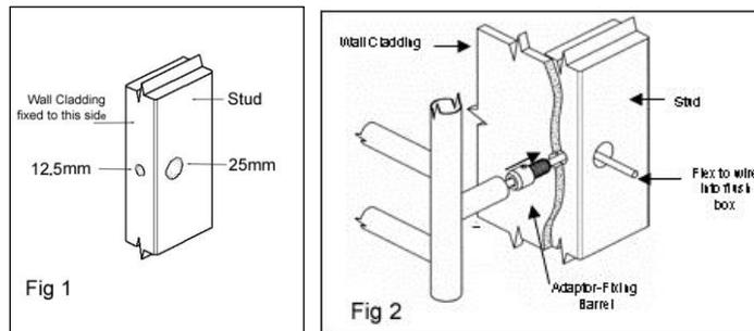
4. Place a pull through line from the flush box and out the 12.5mm hole so that the line can be picked up later once the wall cladding is in place
